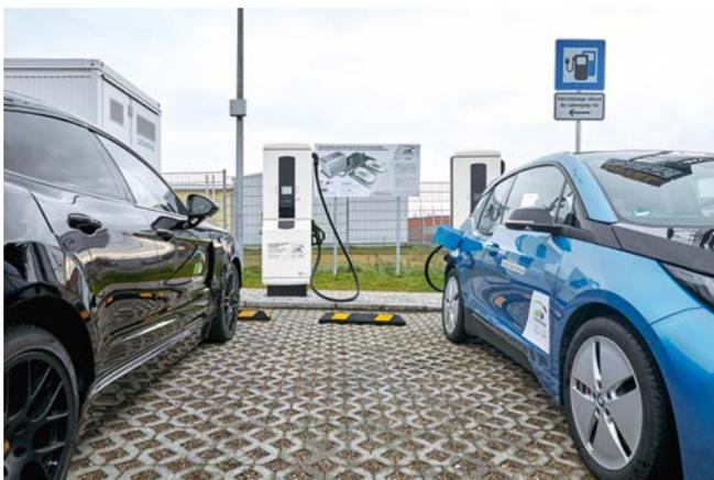
A vital prerequisite for widespread acceptance of electromobility is the ability to charge a vehicle in just a few minutes. The results of a research project at a service area along the A8 highway in Germany show that charging in minutes is now a practical possibility. The cooled HPC charging system from Phoenix Contact plays an important role in this achievement.
