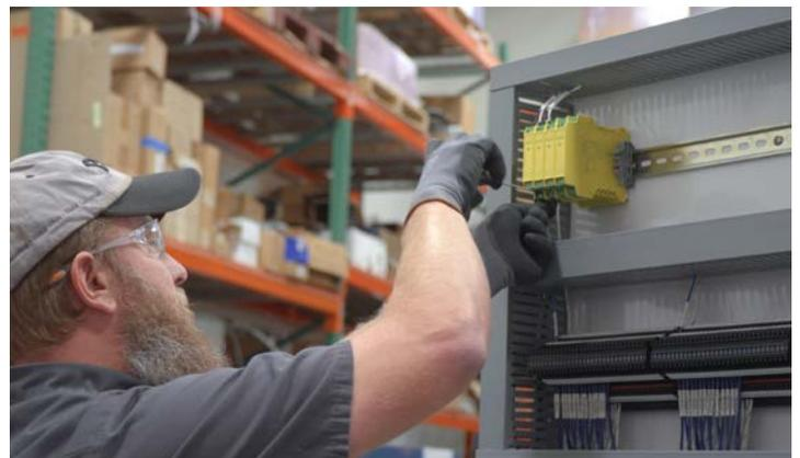
**Figure 3: Safety relays with force-guided contacts are SIL-certified.**
